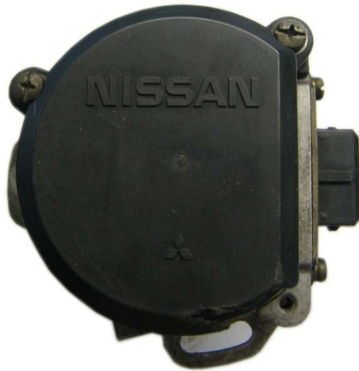
Figure C09.1 - Nissan VH 45 Crank Angle Sensor
