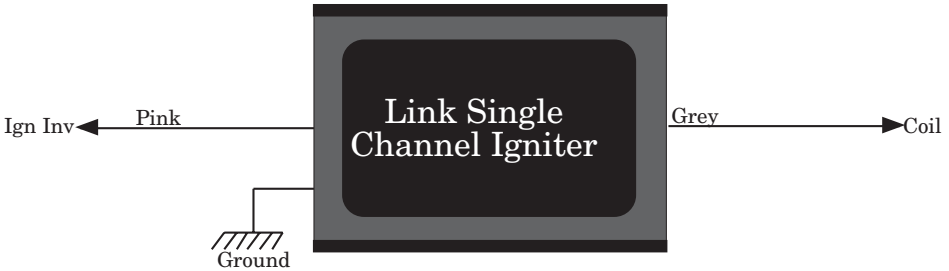
Figure 3.8 (b). Distributor setup with inverted igniter signal (Ign Inv).
