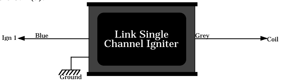
Figure 3.2 (a). Distributor setup with conventional igniter signal (Ign).
