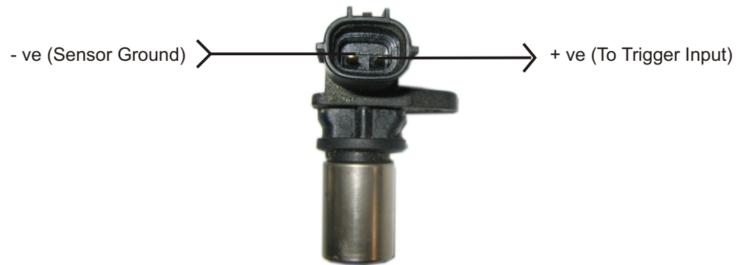
Figure C06.1 - Toyota 1UZFE Crank Angle Sensor Wiring
